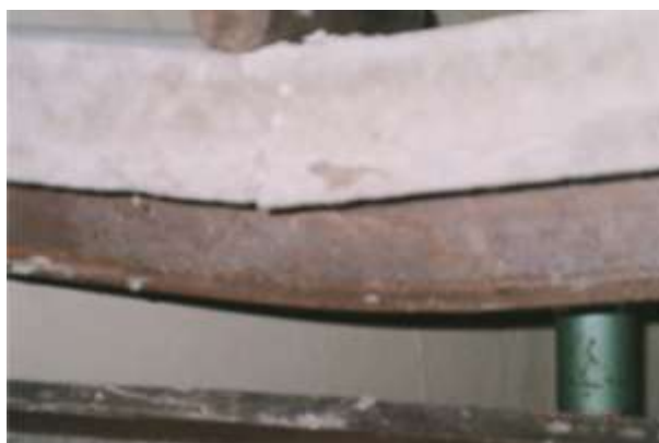
Fig. 9. Failure mode of concrete-steel composite beam.
