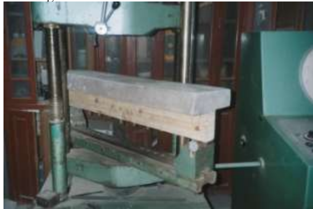
Fig. 5. Test set up for beams.
